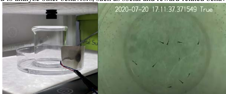
Figure 1. The Raspberry Pi camera is set up to allow recording of zebrafish's startle response during their stimulation. The stimulator is attached to the petri dish wherein a beaker is placed. Larval zebrafish are placed in the beaker directly under the camera. The Pi camera is positioned so that it captures the movement of zebrafish upon the stimulation and save the collected data on Raspberry Pi as a video file. In the second image, the zebrafish are shown mid-response to stimulus.
