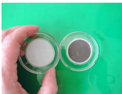
Figure 1: The figure compares the state of two filters with the one on the left being clean and the one on the right after collection of pollution particles.
