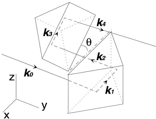
Fig. 1. VAP system for rotating linear polarization by  $\phi$  with right-angle prisms. The angle  $\theta$  between the prisms is varied to change the rotation angle:  $\phi = 2\theta$ . The unitary propagation vectors are  $k_0 = (0, 1, 0)$ ,  $k_1 = (-1, 0, 0)$ ,  $k_2 = (0, -1, 0)$ ,  $k_3 = (-\sin\theta, 0, \cos\theta)$ , and  $k_4 = (0, 1, 0)$ .
