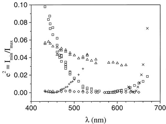
Fig. 5. Measurements of  $e^2 = I_{\min}/I_{\max}$  for a linearly polarized laser beam with an azimuth of  $45^\circ$  reflected off the coated right angle prism (+), coated Ag mirror [New Focus model 5103] ( $\square$ ), dielectric mirror [New Focus model 5102] ( $\times$ ), Al mirror [CVI model PAUV] ( $\triangle$ ) and the VCPS system ( $\diamond$ ).
