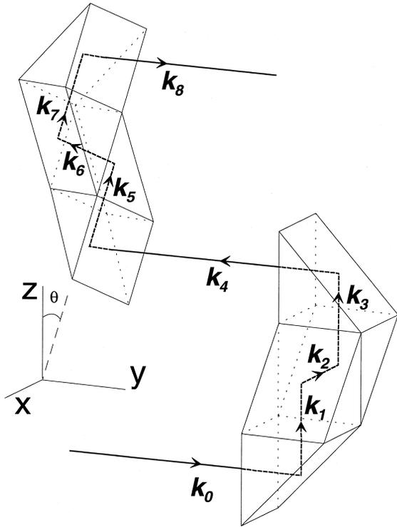
Fig. 3. Schematic of the VCPS system made of cemented right-angle prisms. The unitary propagation vectors are  $k_0 = (0,1,0)$ ,  $k_1 = (0,0,1)$ ,  $k_2 = (-1,0,0)$ ,  $k_3 = (0,0,1)$ ,  $k_4 = (0,-1,0)$ ,  $k_5 = (-\sin\theta,0,\cos\theta)$ ,  $k_6 = (\cos\theta,0,\sin\theta)$ ,  $k_7 = (-\sin\theta,0,\cos\theta)$ , and  $k_8 = (0,1,0)$ .
