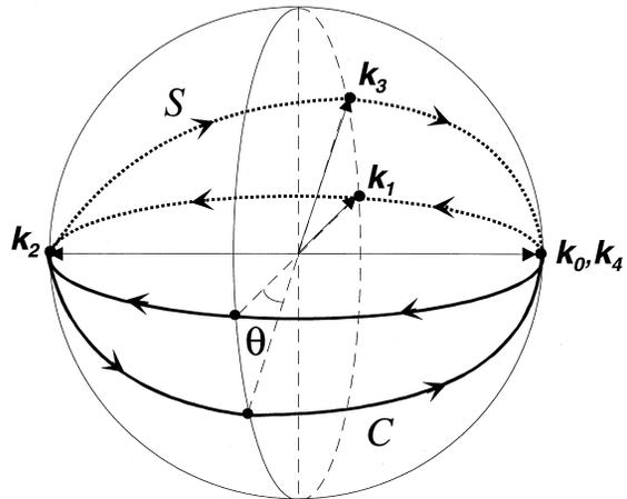
Fig. 2. Mapping of the trajectory of the propagation vector  $k$  ( $S$ ) and helicity vector  $\tilde{k}$  ( $C$ ) for the VAP system. The area enclosed by  $S$  and  $C$  (i.e., the geometric phase) is given by  $\phi = 2\theta$ .
