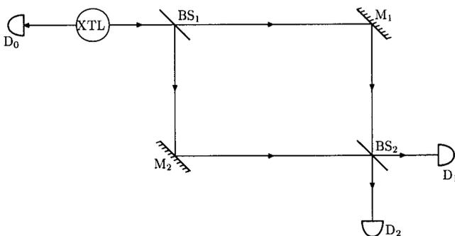
Fig. 2. The motion of the mirror  $M_1$  introduces a phase change in one arm of the Mach–Zehnder interferometer. Interference fringes appear in the counts in  $D_1$  and  $D_2$ . Detection in coincidence with  $D_0$  assures that there is only one photon in the interferometer at the time of detection and, therefore, that a photon interferes with itself.
