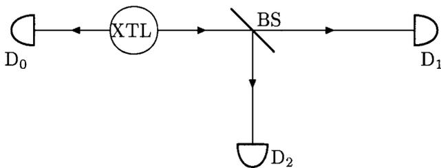
Fig. 1. Two photons emerge from XTL, the down converter—the incident laser beam that excites the down converter is not shown. One photon goes to detector  $D_0$ ; the other goes by way of the beam splitter BS to  $D_1$  or  $D_2$ . The absence of coincidences between detectors  $D_1$  and  $D_2$  demonstrates the existence of the photon.
