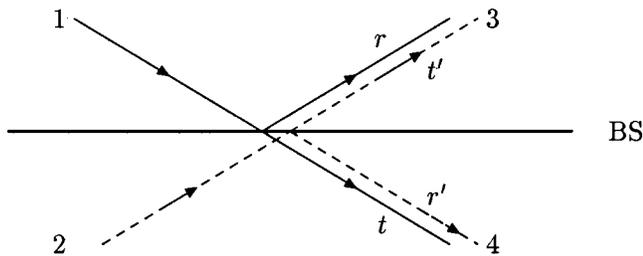
Fig. 4. A schematic representation of an ideal beam splitter with input ports 1 and 2 and output ports 3 and 4. The amplitudes for reflection and transmission from port 1 are, respectively,  $r$  and  $t$ . The corresponding amplitudes for a photon entering 2 are  $r'$  and  $t'$ .
