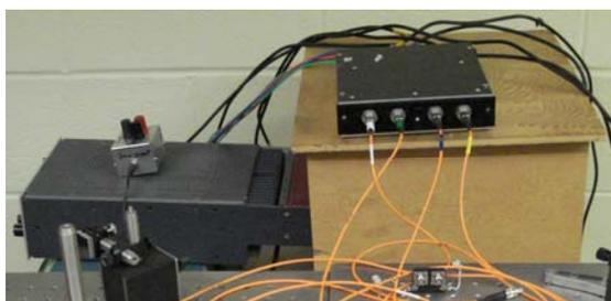
Fig. 11 Fiber-coupled detector module.
