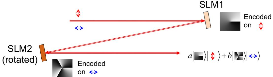
**Figure 5.** Proposed method to encode non separable states of polarization and spatial mode that can allow access to a large Hilbert space. It uses two spatial light modulators (SLM) rotated relative to each other, in reflection mode.
