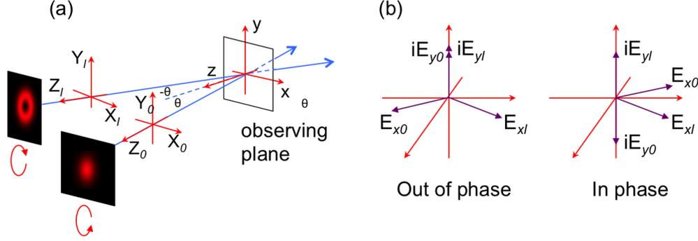
**Figure 1.** (a) Reference frames of the two non-collinear beams and the observing frame. (b) Orientation of the field components at points where the  $x$ -components of the fields of the two beams are out of phase and in phase.
