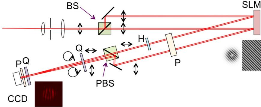
**Figure 4.** Apparatus used to perform the measurements. Optical components include a non-polarizing beams splitter (BS), polarizing beam splitter (PBS), half-wave plate (H), quarter-wave plates (Q), polarizers (P), and spatial light modulator (SLM). Insert shows an example the pattern encoded onto the SLM but with low fringe density for illustration purposes.
