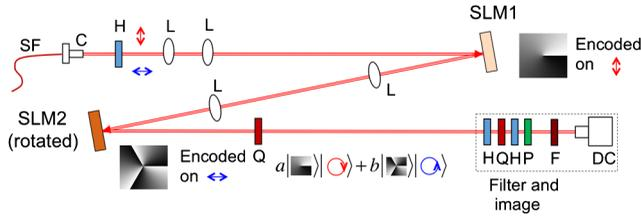
**Fig. 1** Schematic of the apparatus. Optical elements include lenses (L), half-wave plates (H), quarter-wave plates (Q), polarizer (P), neutral density filter (F), single-mode fiber (SF), fiber collimator (C), spatial light modulators (SLM), and digital camera (DC). The SLMs were rotated by 90 deg relative to each other.
