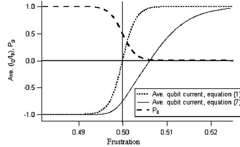
FIG. 3. Normalized average circulating current versus frustration, with finite  $\tau$  [Eq. (7)] and with  $\tau=0$  [Eq. (1)].  $P_0$  is also indicated. The expression that includes finite measurement time is displaced in flux relative to the curve with a fast measurement. The parameters used are  $E_J = 4000$   $\mu$ eV,  $\tau = 100$   $\mu$ s,  $Q = 10^6$ , and  $\alpha = 0.58$ .
