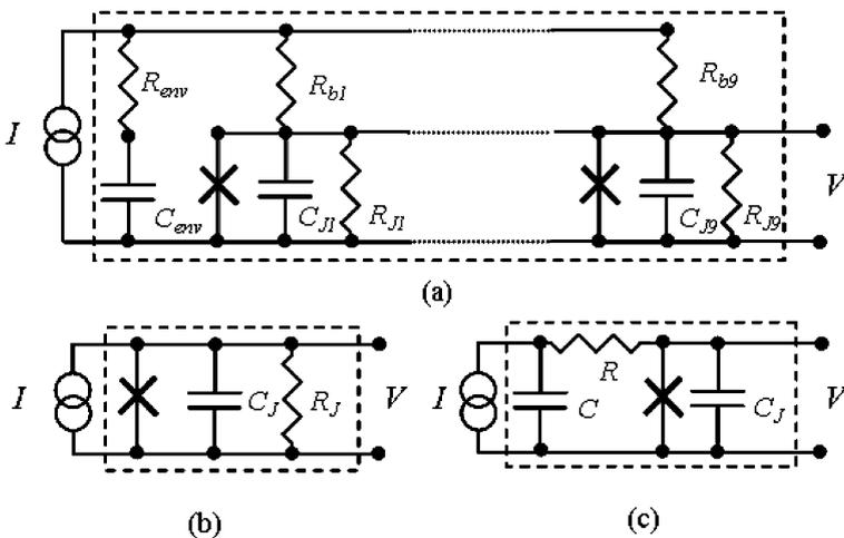
**Fig. 11** Circuit models for the complete array with environmental impedance (a), the typical single-particle picture (b), and the model of Vion et al. (c). The boxes with the dashed lines isolate the measured  $I$  and  $V$ . Note that the resistor and capacitor in model (c) are meant to be part of the array dynamics, not external components
