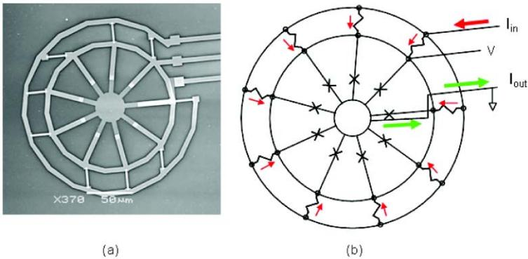
**Fig. 1** Scanning electron micrograph (a) and schematic of the device (b). In the schematic, the junctions are indicated with X's and the application of the current is shown. Red arrows indicate current entering the device while green arrows indicate current leaving the device
