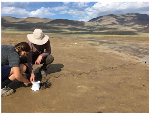
Setting up a station to monitor insolation, temperature, humidity, and soil moisture.
