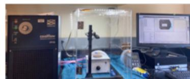
Figure 1: Drop Freeze Apparatus
