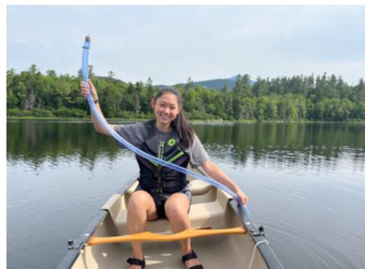
Using an integrated sampler to take a surface sample of a lake
