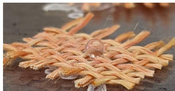
Image B: Drop of water on a 1 cm<sup>2</sup> square of jute, treated with diphenylalanine nanowires to create a hydrophobic surface.
