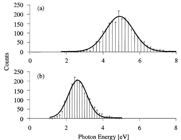
Fig. 3. Histograms of single photon events. Incident photon energies of plot (a) and (b) are  $4.89 \text{ eV}$  and  $2.27 \text{ eV}$ , respectively.
