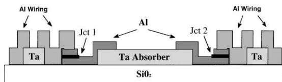
Fig. 1. Schematic of an imaging STJ detector using lateral trapping and backtunnelling. Not shown is an insulating  $\text{SiO}_2$  layer between the trap and wiring.
