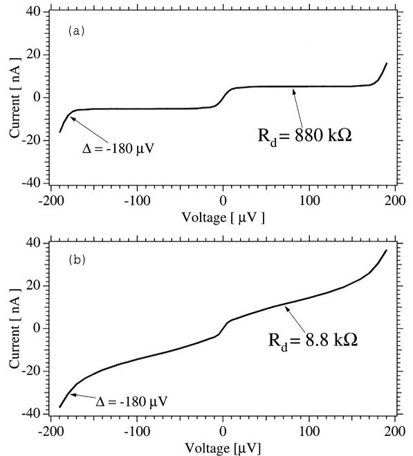
Fig. 2. Subgap  $I$ - $V$  curves of two junctions. Both measurements are made at  $T = 220 \text{ mK}$ . The junction parameters are: (a) area =  $400 \mu\text{m}^2$ ,  $R_{\text{NN}} = 2.3 \Omega$ ; (b) area =  $100 \mu\text{m}^2$ ,  $R_{\text{NN}} = 13.8 \Omega$ .
