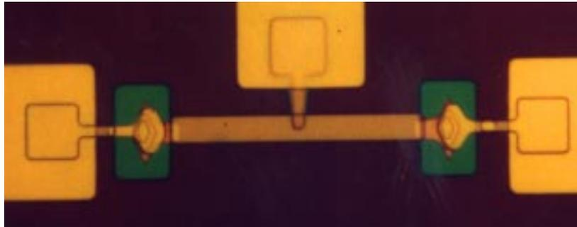
Figure 3. Photograph of the 1-D STJ-based imaging spectrometer tested in optical/UV range.
